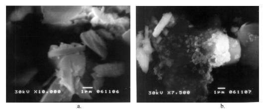
Fig. 2. SEM microphotographs solid residues of concentrate K1, a. spekularit in sulphide-iron basis, 10000×, b. spekularit with gangue minerals magnified 7500×
