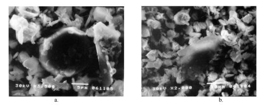
Fig. 4. SEM microphotographs solid residues of concentrate K3, a. sulphur-salts of iron and lead with SiO<sub>2</sub> in center, magnified 2000×, b. sulphur-salts of iron, magnified 3500×
