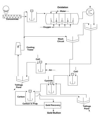
Fig. 1. Diagram of autoclave oxidation with operation stream
