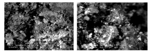
Fig. 3. SEM microphotographs solid residues of concentrate K2 III/18, a. magnified 200×, b. sulphur-salts with SiO<sub>2</sub>, magnified 500×
